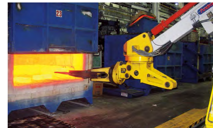
Andromat AMX 40 on a ring forging mill
